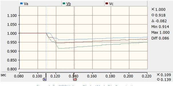
Figure 4-2 - PCC Voltage Dip for Whole Site Energisation
